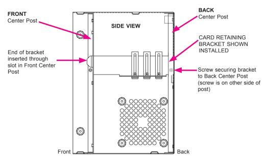
5. Insert the expansion card into the backplane connector and reinstall the screw to secure the card's end plate to the enclosure.
